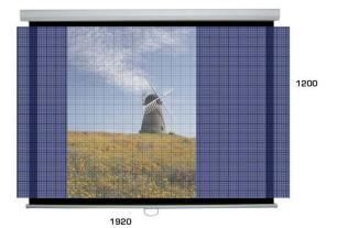
In this image on the right, the 16:10 format image 'grid' is shown, this time in blue, showing a portrait image filling the screen. This should give a guide to how much wider the screen has to be.
