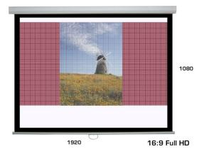
For both **16:9** and **16:10** we have shown the biggest size that pictures can be projected within the resolutions set on the projector (shown as a 'grid').
