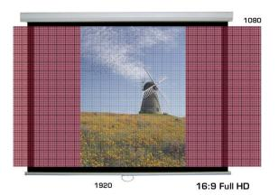
The image on the left shows how much bigger this screen would have to be to fill the screen with a portrait image at 16:9 (image area 'grid' shown in red).
